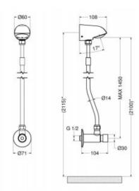
Self-closing shower set with a fixed spout mounted to the wall. The supply pipe has a diameter of 14 mm and, what is important, the mounting is fitted to wall mounting. The shower set has one 1/2 &HASH39; connection for cold or mixed water, with a standard water flow time of about 30-50 seconds ± 1 second. The flow system is enriched with a safety device that automatically shuts off the water flow after 15 seconds (at a pressure of 3 bar).
