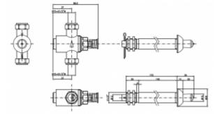
Shower tap for concealed installation. The tap has one G1 / 2 connection for cold or mixed water. The body of the faucet is made of brass. A single outflow of water in the 9005 shower tap takes about 15 - 25 seconds. The amount of water consumed at the outlet is approx. 6 l / m, at a water connection pressure of 3 bar. The connection pressure can be from 0.5 to 6 bar, however, the recommended connection pressure should be from 2 to 4 bar.
