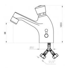
The washbasin timer with an integrated mixer and aerator a reliable product most often used in public spaces. The 9007 faucet is made of corrosion-resistant chrome-plated brass. In the side part of the body there is a mixer, regulated by a lever.
