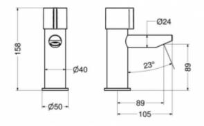
A time button faucet made of chrome-plated brass is a device adapted to public spaces - including hotels, shopping malls, public toilets, and others. The 9008 faucets is equipped with two 1/2 &HASH39; connections for cold and hot water. In the upper part of the body, there is a built-in mixer, thanks to which the user can freely change the water temperature.
