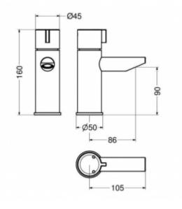
The 9008T button thermostatic time battery is made of chromeplated brass and is perfect for public use. The offered faucet has a built-in mixer so that the user can change the water temperature on his own. What&HASH39;s more, the 9008T model uses a modern TMV3 thermostatic expansion valve. TMV series valves are used in general refrigeration, they are used in devices with one or more cooling circuits.
