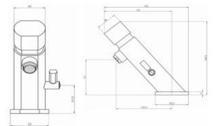
The washbasin timer with an integrated mixer and strainer is a reliable product most often used in public spaces. The 9077 faucet is made of corrosion-resistant chrome-plated brass. In the side part of the body, there is a mixer, regulated by a lever. There is a strainer in the spout that regulates the water stream.
