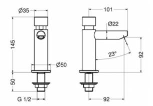
The self-closing basin tap with a moving aerator. The body is made of chrome-plated brass. The tap has one G1 / 2 connection. A single outflow of water takes about 15 seconds (at a water pressure of 3 bar). The amount of water used is 5 l / m. The minimum connection pressure is 1 bar, the maximum is 5 bar. It is worth adding that the recommended connection pressure should be 2-4 bar.
