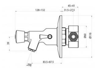
Washbasin timer with a manual mixer in the form of a lever located on the side of the faucet, which makes temperature regulation easy and more under control.
