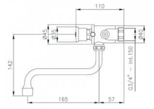
A self-closing tap with a mixer and a movable spout is a universal product that is perfect for public use. Thanks to the use of a movable spout, the 9092L mixer can be used with twocompartment sinks. Moreover, the mixer is equipped with levers that facilitate operation, e.g. for the disabled or for children. The fittings has two 3/4 "connections for hot and cold water. The body is made of chrome-plated brass and has a 15-year warranty.
