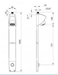
Self-closing shower panel with G1/2 connection for cold or mixed water. It is possible to connect the water supply from the top - at the head, or from the wall. The faucet head is made of brass, while the rest of the panel is made of durable plastic and aluminum.
