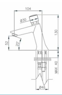
The washbasin timer with an integrated mixer and aerator a reliable product most often used in public spaces. The 9777 faucet is made of corrosion-resistant chrome-plated brass. In the side part of the body there is a mixer, regulated by a lever.
