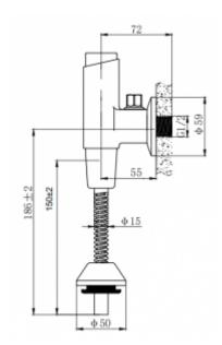
A urinal set is a functional product that is made of durable brass covered with a chrome layer. The offered set has one connection 1/2&HASH39;&HASH39; for cold or mixed water. The set can be started by press the button. Possible water flows time is 7 seconds +/- 3, with pressure 0.5 - 6 bar range. The offered set is perfect for public places such as swimming pools, saunas, shopping malls, offices, hotels, etc.
