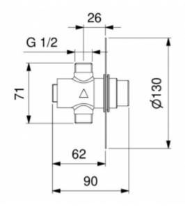
Flush-mounted urinal time valve. Designed for flush mounting, making it fully resistant to vandalism. Used for flush-mounted urinals.
