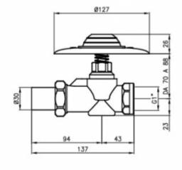
WC timer, floor. Intended for toilet bowls with concealed supply or other toilet intakes. Thanks to the floor installation, the flushing machine is ideal for people with disabilities. The button located on the floor has a cover made of thick rubber, thanks to which it is protected against dirt and vandalism.
