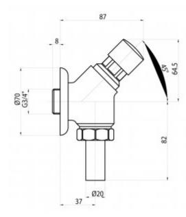
Surface-mounted toilet timer. Designed for toilet bowls with surface-mounted supply. The button located at an angle of 45 ° significantly facilitates the use of the flushing valve. Equipped with anti-impact system eliminating "hydraulic shock" when closing the valve.
