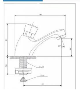
Washbasin time tap with one G1/2 connection, for cold or mixed water. The faucet body is made of brass covered with a chrome layer. There is an aerator in the spout. A single flow of water during start-up lasts 7 seconds +/- 3 seconds. The working water pressure is from 1 to 6 bar. The water temperature range can be  $0 - 50 \square$ . The offered 9101 battery is available in three variants:
