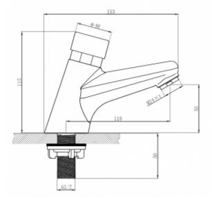
Washbasin time tap with one G1/2 connection, for cold or mixed water. The faucet body is made of brass covered with a chrome layer. There is an aerator in the spout. A single flow of water during start-up lasts 7 seconds +/- 3 seconds. The working water pressure is from 1 to 6 bar. The water temperature range can be  $0 - 50 \square$ . The offered 9102S tap is available in two variants:
