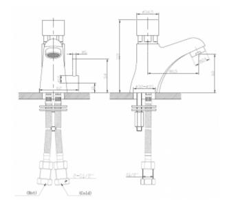
The washbasin tap with a build-in water mixer is with two flexible connections G1 / 2. The faucet body is made of corrosion-resistant chrome-plated brass. A single flow of water during start-up lasts 7 seconds +/- 3 seconds. The working water pressure can be from 1 to 6 bar. The water temperature range is 0 - 50  $\square$ . The tap has a built-in aerator. In addition, check valves and strainers are included in the set.
