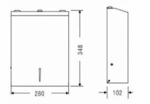
Paper towel dispenser made of stainless steel.Polished finish. Capacity: 400-600 ZZ folded towels. Lockable with a key. Ground edges. Distribution: 1 paper towel. It has a window for viewing the remaining amount of paper.
