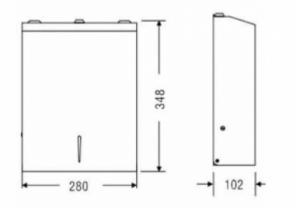
Paper towel dispenser made of stainless steel. Matte finish. Capacity: 400-600 ZZ folded towels. Lockable with a key. Ground edges. Distribution: 1 paper towel. It has a window for viewing the remaining amount of paper.
