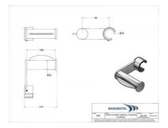
Toilet paper holder - polished or matte. The holder is adapted to be mounted on handrails with a thickness of Ø32.
