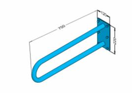
Handrail for disabled people, arched, fixed, 700 mm long, generalpurpose, made of 32 mm diameter carbon steel tube, white powder coated. We use this type of handrail in the washbasin, shower, and toilet area.
