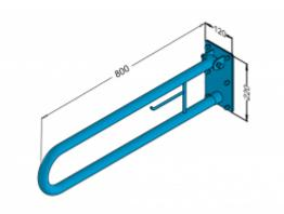
Handrail for disabled people, arched, tilted, wall with space for toilet paper, 800 mm long, general purpose, made of 32 mm diameter carbon steel tube, powder coated, white. We use this type of handrail in the wc area.
