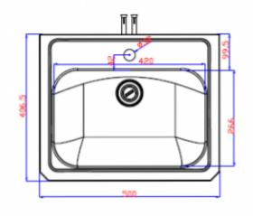
Stainless steel washbasin, suspended. Has good shape and effective looks. Designed for montage standing sink batteries.
