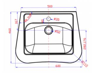
The safe SB16 washbasin made of AISI 304 stainless steel is a key product that is the perfect complement to commercial bathrooms for the disabled. It is worth mentioning here that the AISI 304 steel used for production is characterized by high resistance to moisture, rust, corrosion, and also to some acids.
