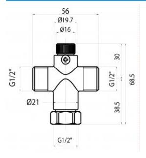
Under-basin mechanical mixer. Used in wash basin fittings serving one water.
