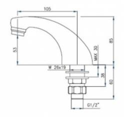
Riser-type washbasin spout with one G1 / 2 connection. The spout&HASH39;s body is made of brass with a layer of chrome. An aerator has been installed at the point of water outflow. The maximum water outflow force may be 21 l/m at a pressure of 3
