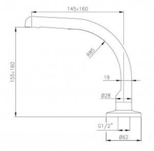
Riser-type washbasin spout with one G1 / 2 connection. The spout&HASH39;s body is made of brass with a layer of chrome. An aerator has been installed at the point of water outflow. The maximum water outflow force is 21 l/m at a pressure of 3 bar. The water connection temperature can be between 5  $^{\circ}$  C and 65  $^{\circ}$ C. On the other hand, the water connection pressure can range from 0.5 - 6 bar, while the recommended connection pressure should be 2-4 bar.
