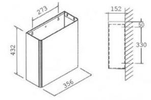
Open basket made of stainless steel. Matte finish. Vandal resistant design. Capacity: 25 L. Wall mount. The basket is equipped with hooks for securing the bag. High quality stainless steel: AISI 304, 1.2 mm.
