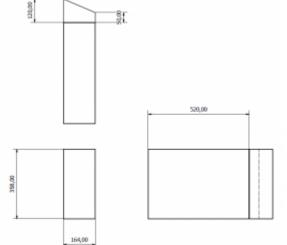
Basket with a hinged lid made of stainless steel. Matt finish. Vandal resistant design. Capacity: 28 L. Wall mount. The basket is equipped with hooks for securing the bag. High quality stainless steel: AISI 304, 1.2 mm.
