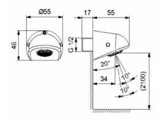
Shower spout with movable strainer. Made of chrome-plated brass. Adapted for flush mounting. The spout makes it resistant to vandalism. The slim design definitely makes it difficult for the user to devastate the screed by hanging on it, which may result in the screed being pulled out. The strainer has a cover made of rubber, which makes it easier to maintain and less exposed to limescale.
