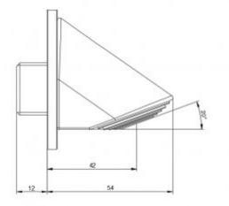
Solid spray spout. Made of chrome-plated brass. Adapted for flush mounting. It has an unregulated angle of water jet of 16 degrees. The spout makes it resistant to vandalism. The slim design definitely makes it difficult for the user to devastate the screed by hanging on it. Recommended for mounting on campsites, baths, swimming pools, schools, gyms and fitness clubs.
