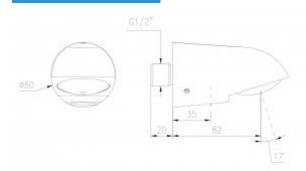
Solid spray spout. Made of chrome-plated brass. It is distinguished by the possibility of using it for installation in surface or flushmounted versions.
