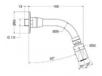
Shower spout with a movable head. Made of chrome-plated brass. Adapted for flush mounting. Thanks to the extension in the form of a tube, the spout is moved away from the wall, which allows the shower to be used at a greater distance from the wall. The angle of the water jet can be adjusted.
