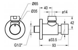
The shower timer valve is a product made of AISI 316L stainless steel for wall mounting. The valve can be actuated using a button located in the central part of the device, moreover, the valve has a water flow system that automatically closes after 15 seconds (at a pressure of 3 bar). What&HASH39;s more, the valve has one 1/2 &HASH39; connection for cold or mixed water. Valves such as 9004INOX are most often used in places with only devices suitable for surface water supply.
