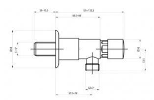
Urinal time valve for cold water. Used for wall mounting. Equipped with a water flow pressure regulator reducing water consumption to 6l / minute
