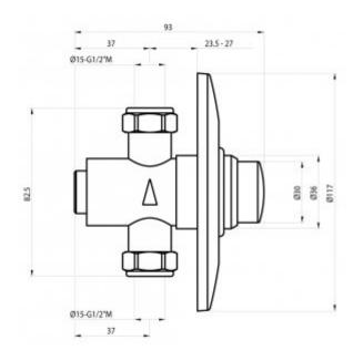
Flush-mounted urinal time valve. Designed for flush mounting, making it fully resistant to vandalism. Used for flush-mounted urinals.
