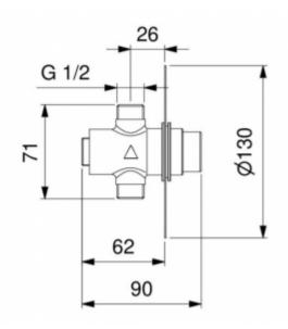
Flush-mounted urinal time valve. Designed for flush mounting, making it fully resistant to vandalism. Used for flush-mounted urinals.
