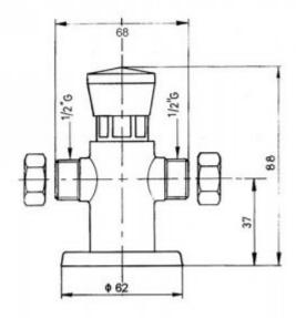
Shower tap for concealed installation. The tap has one G1 / 2 connection for cold or mixed water. The body of the faucet is made of brass covered with a layer of chrome. A single outflow of water in the 9006 shower tap takes about 15 - 25 seconds. The amount of water consumed at the outlet is approx. 6 l / m, at a water connection pressure of 3 bar. The connection pressure can be from 0.5 to 6 bar, however, the recommended connection pressure should be from 2 to 4 bar.
