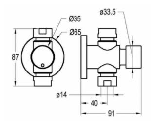
Shower timer for exposed installation. Most often used in places with only devices adapted to surface water supply. Self-closing time 15 secs at 3 bars (not adjustable). The body of the shower timer is made of AISI 316 stainless steel with brushed external parts.
