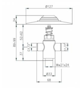
Concealed floor-mounted self-closing pedal tap for general use. The faucet consists of a body made of brass, with a chrome plate and a water flow switch covered with black rubber. The 9009 time battery has one G1 connection for cold or mixed water and one G1 / 2 connection. One rush of water takes about 6 seconds ± 2 seconds. The amount of water consumed is approximately 12 l / m at a working water pressure of 3 bar.
