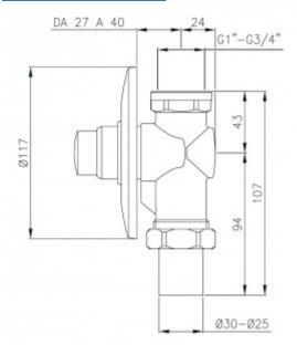
WC timer, concealed. Designed for toilet bowls with concealed supply. Equipped with anti-impact system eliminating "hydraulic shock" when closing the valve.
