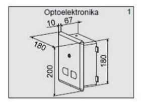
Electronic WC photocell battery. Designed for montage directly to pressure installation. Designed for public facilities.
