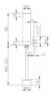
Touchless urinal mixer powered by  $4 \times 1.5 \text{V}$  AA Lithium, designed for wall mounting. The water flow is activated by a photocell, it does not require manual operation by the user. The touchless, urinal mixer is equipped with one 1/2 &HASH39; connection for cold or mixed water. The body is made of brass covered with chrome.
