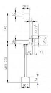
Touchless urinal mixer powered by 4 x 1.5V AA Lithium, designed for wall mounting. The water flow is activated by a photocell, it does not require manual operation by the user. The touchless, urinal mixer is equipped with one 1/2 &HASH39; connection for cold or mixed water. The body is made of brass covered with chrome.
