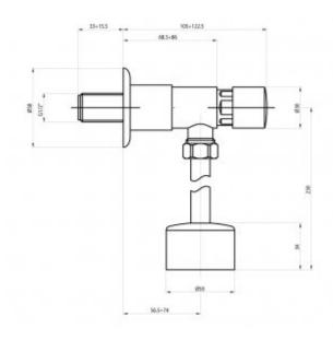
Urinal time set for cold water. Used for wall mounting. The ideal solution for urinals with external power supply.
