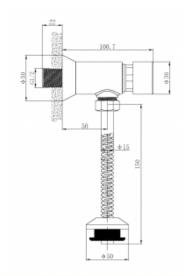
A urinal set is a functional product that is made of durable brass covered with a chrome layer. The offered set has one connection 1/2&HASH39;&HASH39; for cold or mixed water. The set can be started by press the button that is located in the central part of the device. Possible water flows time is 7 seconds +/- 3, with pressure 0.5 - 6 bar range. The offered set is perfect for public places such as swimming pools, saunas, shopping malls, offices, hotels, etc.
